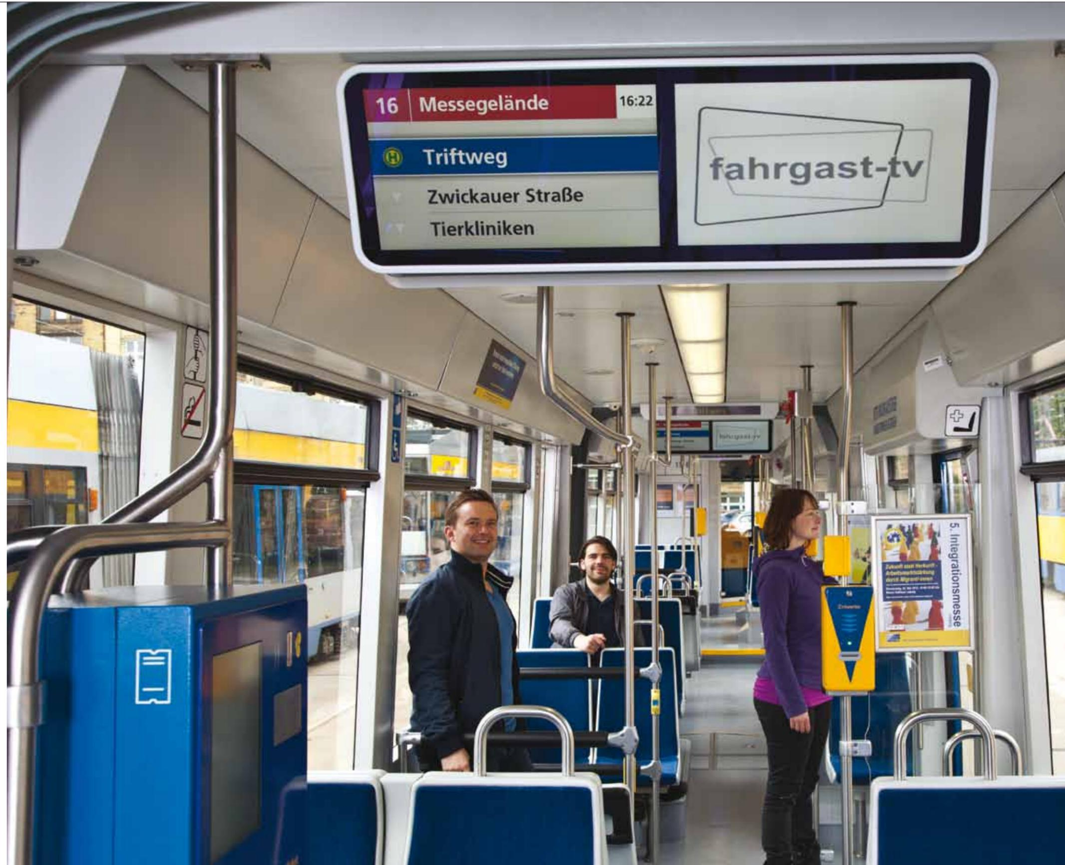
“The GigaSTaR technology also supports long distances between the displays and ensures a robust signal transfer between the cars,” says Kreidl. “In addition, all parameters like temperature and display functions are monitored, and this information is automatically transferred so operators can see when a unit needs to be serviced.”
